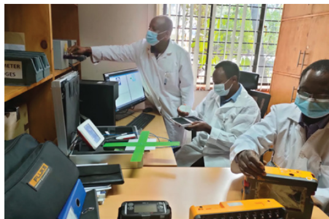
CHAK HCTS technical team in the Dosimetry Lab working on dosimetry reading for radiation monitoring badges and New Fluke Gas Flow Analyzer for Anaesthesia equipment calibration and quality assurance, all acquired from Germany through support by BfdW.
